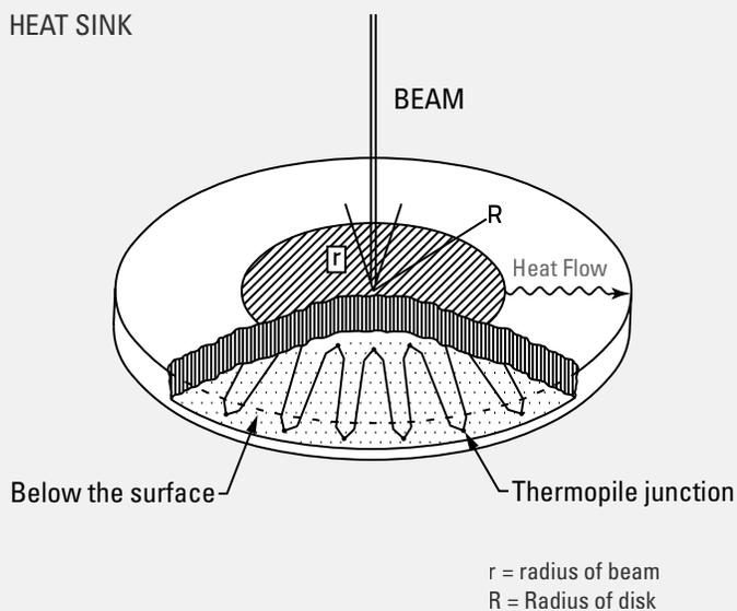
Figure 1. Disk type thermopile
